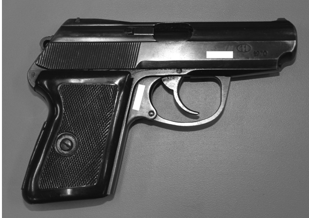
Figure 5.11 A Polish P64 pistol, based on the Walther PP. The year of manufacture is 1970; the arsenal is indicated by the circle 11 icon, indicating production by the Radom Arsenal. (Image from author's collection.)
